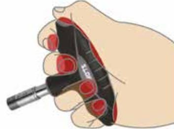
The T-Flying handle is needed whenever particularly high torque for loosening or tightening jobs needs to be applied.
